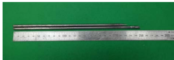
Fig. 1. Typical U-10Zr-10RE fuel slug fabricated with the injection casting process under modest pressure.
