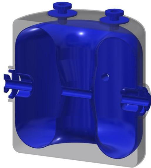
Fig. 1. Superconducting half wave resonator.
