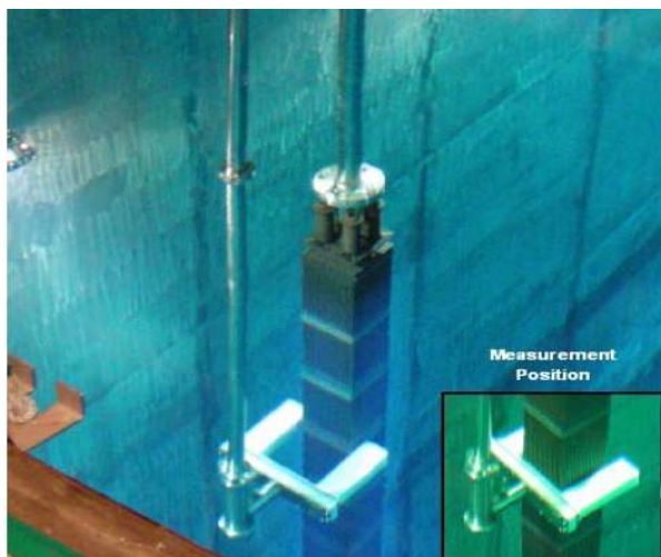
Fig 2. Fork Detector Irradiated Fuel Measurement [1]
