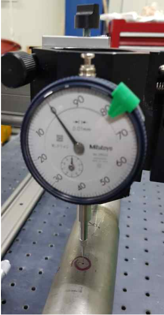
Fig. 1. Devices to measure the heat flux and the hole depth of 24 holes for TC installation.
