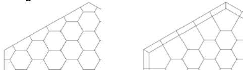
Fig. 1. Chopped Model and Elongated Model for the modeling of residual regions between pin cells and assembly boundaries.
