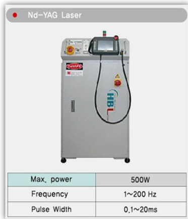
Fig. 2. LBW system used in this experiment.
