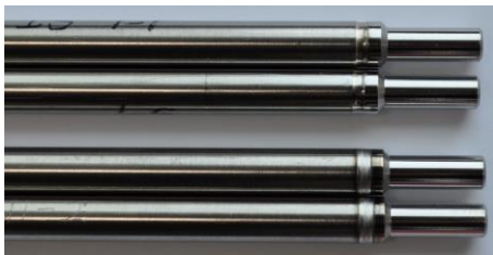
Fig. 3. The weld specimen prepared by LBW.
