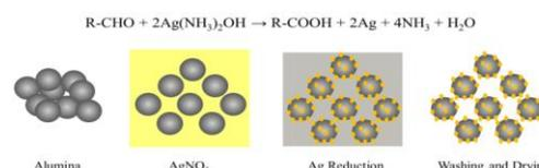
Fig. 2. Synthesis of silver-adsorbed alumina using ascorbic acid and the silver mirror reaction. In the case of Method 1, silver nitrate is mixed with acidic alumina, and the surface silver is reduced by using ascorbic acid in the presence of silver nitrate on the alumina surface. In the case of Method 2, silver is adsorbed on the surface of alumina while silver is reduced using reducing sugar while spherical alumina is stirred in a solution together with silver nitrate.
