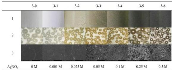
Fig. 3. (1), (2) Color of silver-adsorbed alumina (spherical) as a function of AgNO<sub>3</sub> concentration (silver mirror reaction). (3) SEM images of Ag NPs on the alumina surface. As the concentration of silver nitrate increases, the color of silver-adsorbed alumina (spherical) gradually increases (1), and it is confirmed by optical microscope (2). Silver nanoparticles adsorbed on the alumina surface increase in size and become larger (3).
