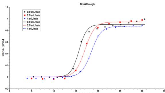
Fig. 4. Breakthrough curve. ● is measured every 2 minutes when the sample was passed through the column at 0.9 mL/min. ■ is measured every minute when the sample was passed through the column at 2.5 mL/min, and ◆ is measured every 30 seconds at 4 mL/min.
