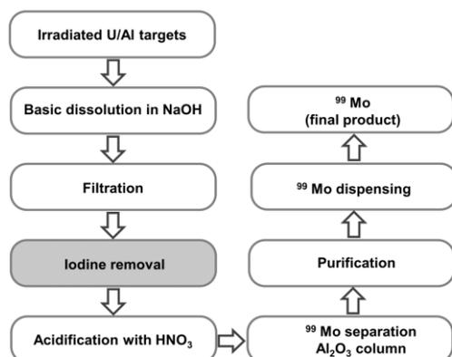
Fig. 1. Overall scheme of <sup>99</sup>Mo production. After dissolving the target with a strong base solution, filter the metal impurities. For purification of <sup>99</sup>Mo, the iodine present in the solution must be removed before the solution is acidified.
