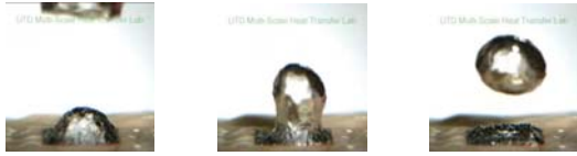
(c) Vapor mushroom behavior of the heat transfer experiment with hydrophobic surface condition at CHF trigger [15].
