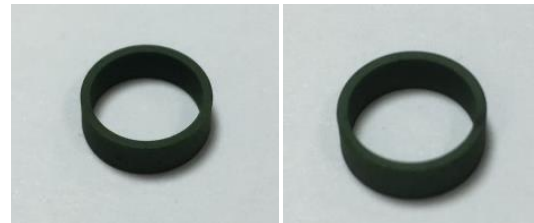
Fig. 5. The Cr and Cr-alloy coated Zircaloy-4 after high temperature steam oxidation tests.
