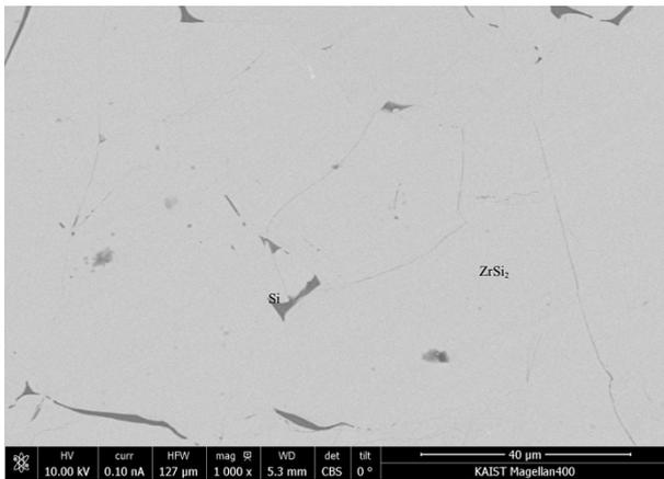
Figure 2. Microstructure of sample 2
