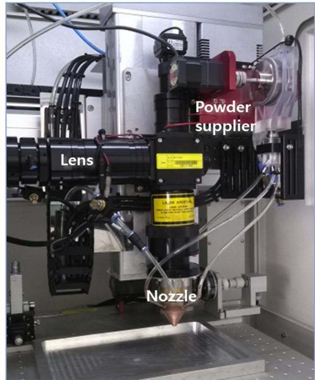
Figure 4 Appearance of the laser cladding equipment [4]
