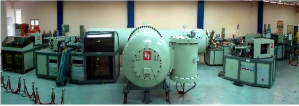
Fig. 1. 3-MV tandem accelerator at Seoul National University
