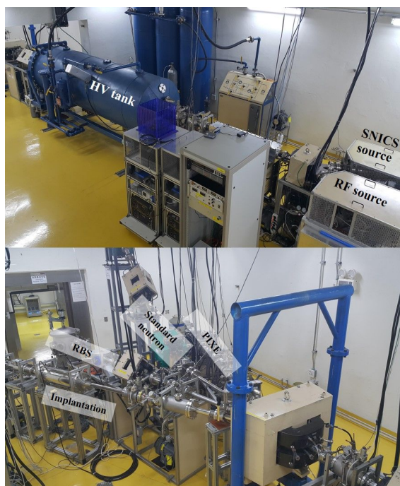
Figure 1. 1.7 MV tandem accelerator at KOMAC
