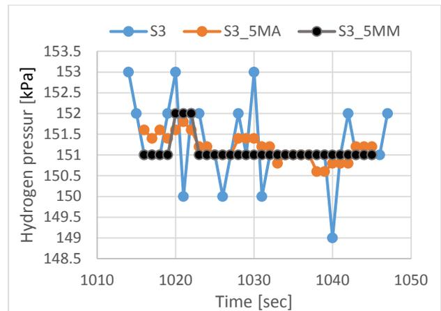
Figure 1. Difference between MA and MM filters applied on one hydrogen transmitter data (S3).
