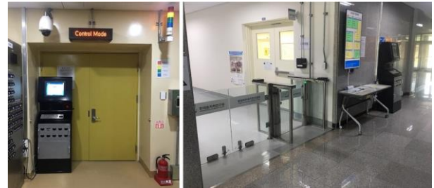
Fig. 6 the EPD readers which would have being installed at the entrance of the radiation controlled area respectively in the acceleration building and ion beam application building.
