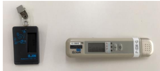
Fig. 2 The thermo-luminescence dosimeter (left) and electric pocket dosimeter (right) used as the main and secondary dosimeter in the radiation controlled of the KOMAC, respectively.
