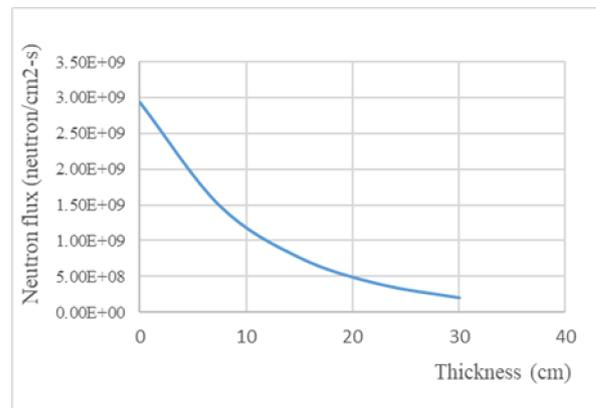
Fig. 2 Neutron distribution in concrete
