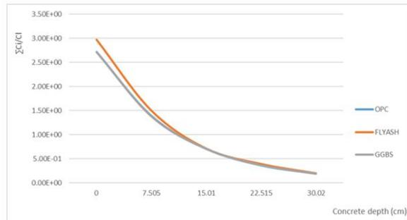
Fig. 3. Concentration ratio against concrete thickness
