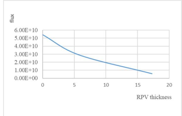
Fig. 1. Neutron attenuation in RPV
