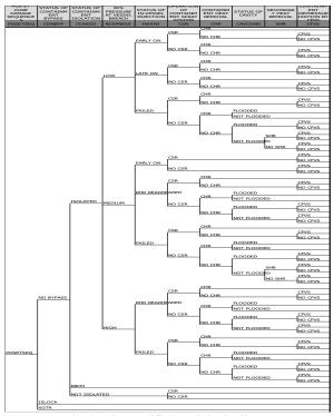
Fig. 2. The modified PDS logic diagram
