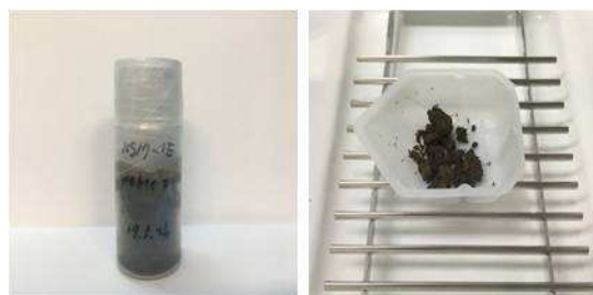
Fig. 1. Concrete sample mixed with processed liquid waste
