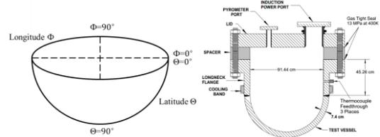
Fig. 1. Schematics of the OLHF experiment [2]
