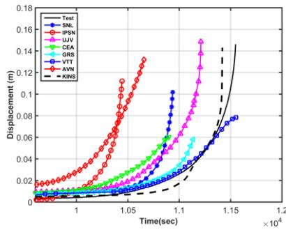
Fig. 7. Vertical displacement at the ex-vessel wall ( $\theta = 90^\circ$ ,  $\varphi = 0^\circ$ )
