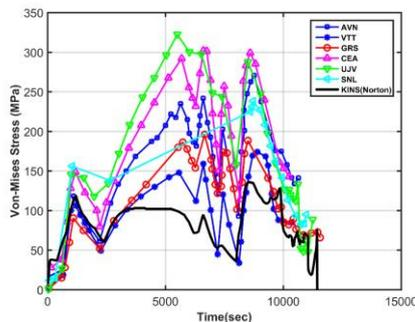
Fig. 9. Von-Mises stress at the ex-vessel wall. ( $\theta = 90^\circ$ ,  $\varphi = 0^\circ$ )
