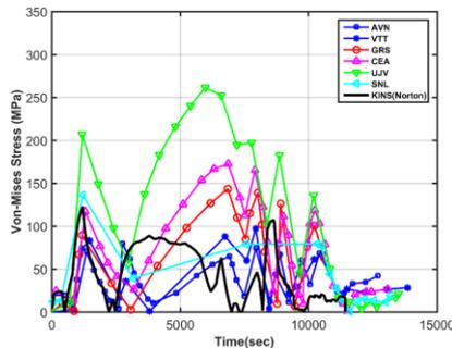
Fig. 8. Von-Mises stress at the in-vessel wall. ( $\theta = 90^\circ$ ,  $\varphi = 0^\circ$ )
