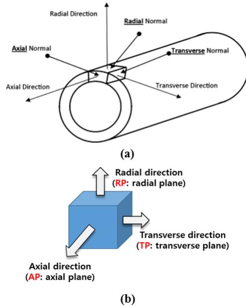
Fig. 1. Schematic diagram of PT. (a) main directions and (b) main planes.
