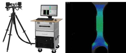
Fig. 2. Digital image correlation (DIC) system and the calculated strain distribution during tensile test.
