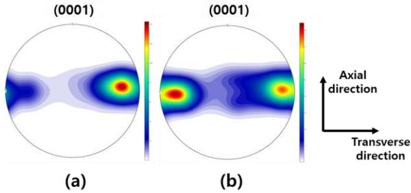
Fig. 3. (0001) basal pole figure of (a) back-end and (b) front-end PT material.
