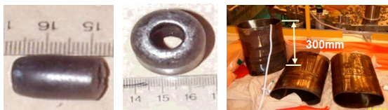
(a) Pins (b) Nuts (c) Thermal Sleeves Figure 1. Examples of the loose parts
