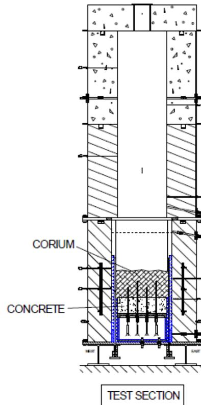
Fig 1. CCI-6 test apparatus [1]
