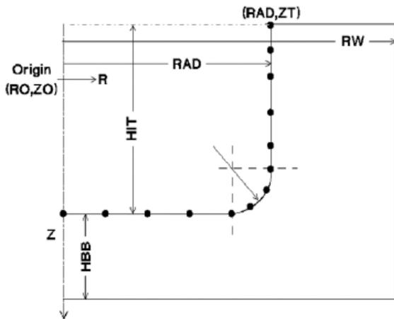
Fig 2. Cavity shape in MELCOR simulation [3]
