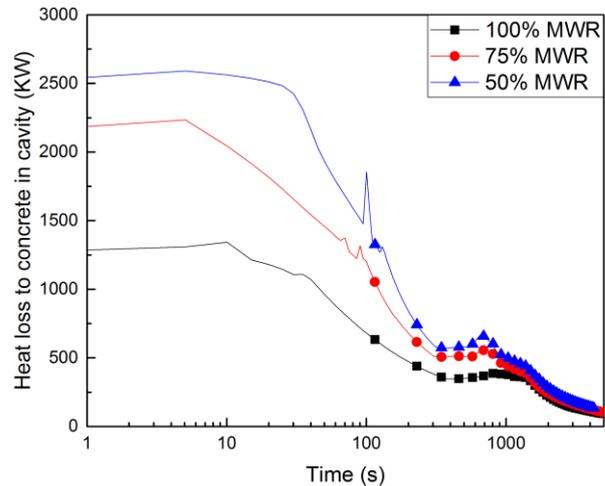
Fig 3. Heat loss to concrete in cavity for each case
