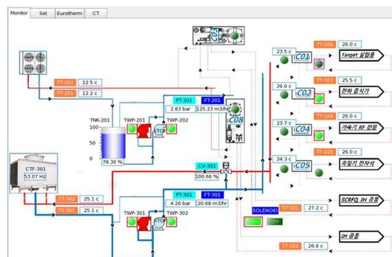
Fig. 1. Monitoring Tab for DIAC cooling system
