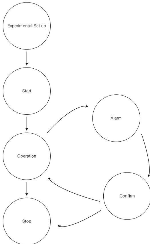
Fig. 3. State transition diagram of the DIAC cooling System
