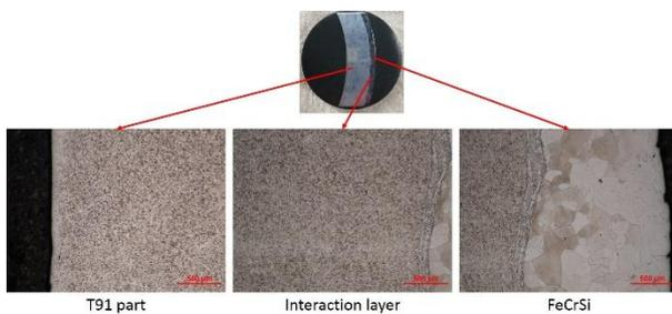
Fig. 1 Optical Microscopy image for OD clad T91 specimen
