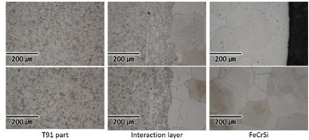
Fig. 2 Optical Microscopy image for OD clad T91 specimen
