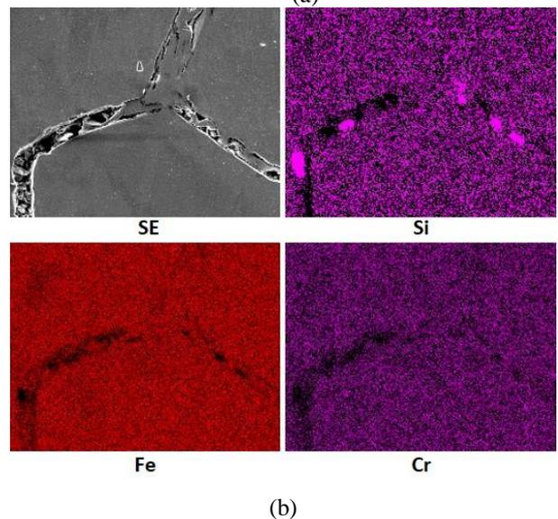
Fig. 3 (a) SEM image for crack on OD clad T91 (b) EDS mapping image for crack on OD clad T91
