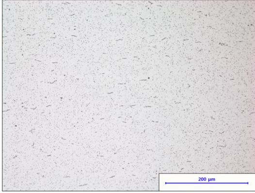
Fig. 1. Micrograph of as received (Case I) Zr-2.5wt%Nb alloy obtained by the optical microscope( $\times 200$ ). The hydrogen concentration is 12 ppm.
