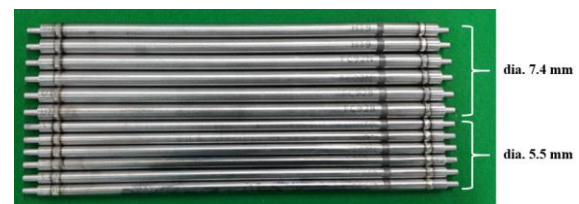
Fig. 5. Photograph of fuel rodlets after welding of endcaps.
