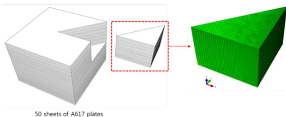
Fig. 1. Diffusion bonding specimen and analysis domain.
