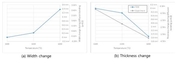
Fig. 5. Permanent dimensional change of diffusion-bonded specimens at various temperature.
