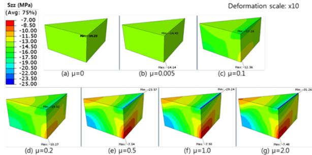
Fig. 4. Normal stress in z-direction at the end of diffusion bonding (1150°C).
