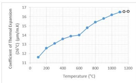
(c) Coefficient of thermal expansion (@26°C)
