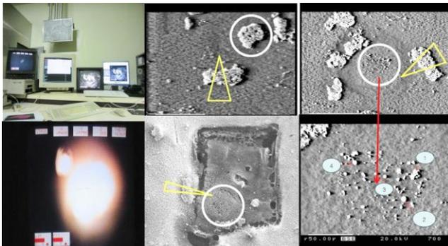
Fig. 2. EPMA monitor, burning spot on monitor, crud flake before and after burning. (20 kV, 1200 nA, beam exposure time; 5 s)
