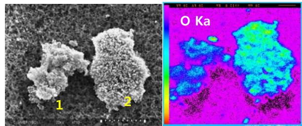
Fig.1. SEM and x-ray map of a crud flake (applied to normal beam current injection).
