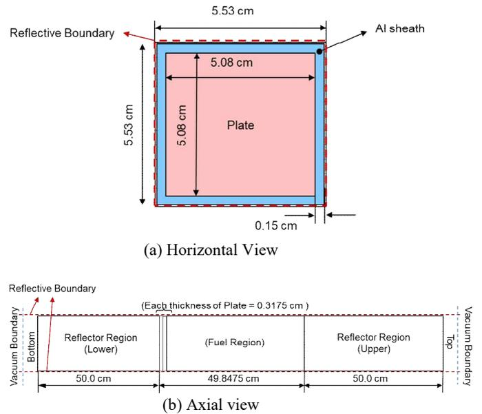
Fig. 1. Overview of the target assembly model.
