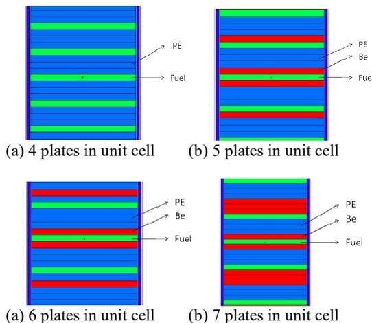
Fig. 4. Fuel assemblies designed by AADP.
