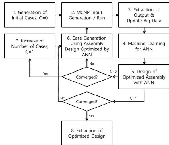
Fig. 3. Overview of automatic design algorithm of the fuel assembly including ANN and machine learning.
