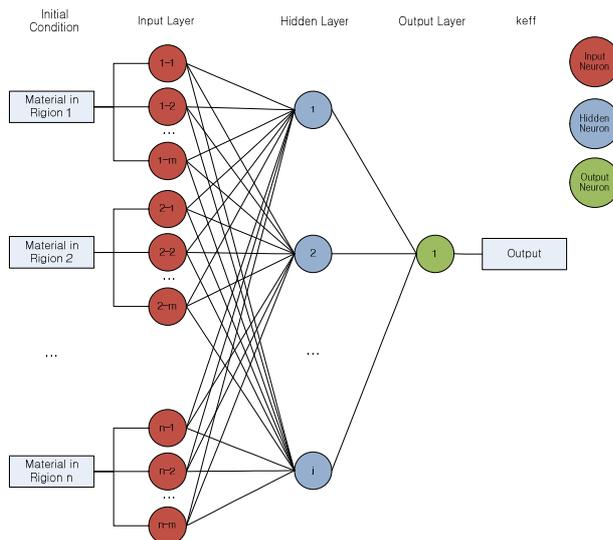
Fig. 2. Feedforward neural network for design of fuel assembly [2].
