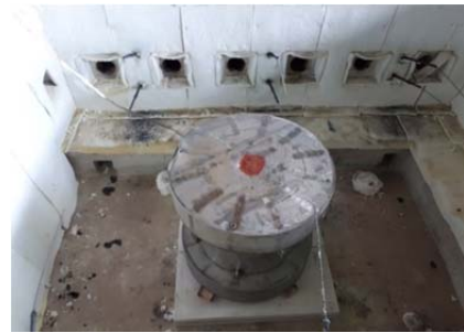
Fig. 2. Half scale model installed in the furnace
