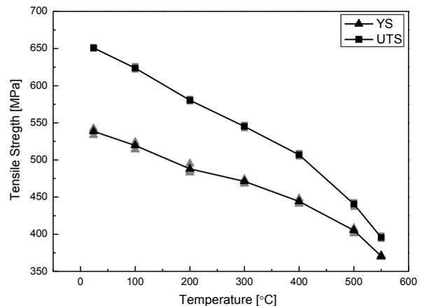
Fig. 4 Tensile strength of ARAA with temperature after PWHT at  $730^{\circ}\text{C}/1\text{h}$ .
