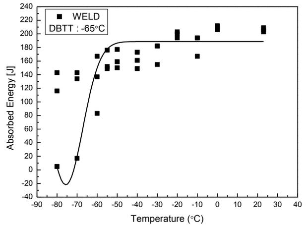
Fig. 3 Results of the Charpy impact test on the WM of the TIG welding joint of an ARAA plate after PWHT at  $730^{\circ}\text{C}/1\text{h}$ .
