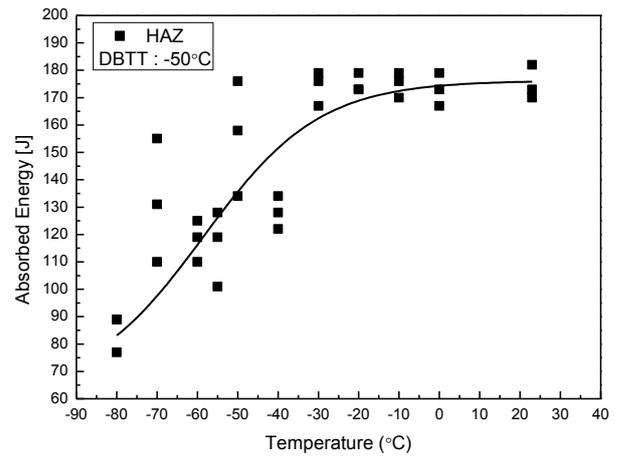
Fig. 2 Results of the Charpy impact test on the HAZ of the TIG welding joint of an ARAA plate after PWHT at  $730^{\circ}\text{C}/1\text{h}$ .
