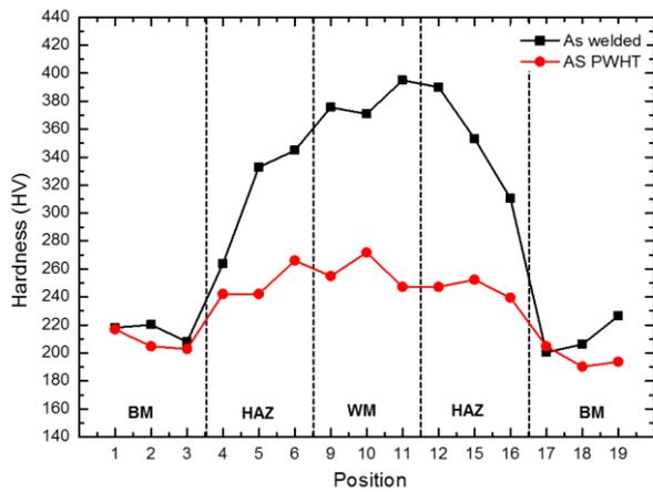
Fig. 1 Results of hardness test across the TIG welding joint of an ARAA plate before and after PWHT at  $730^{\circ}\text{C}/1\text{h}$ .
