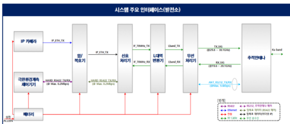
Fig. 2. Interface between components located at NPP
