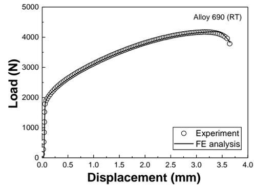
Fig. 4. Comparison of L-d curves from FE analysis and test
