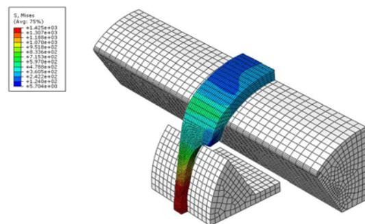
Fig. 3. FE model for simulation of circumferential tensile test
