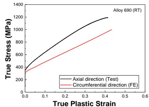
Fig. 5. True stress-true plastic strain curves for axial direction from the test and for circumferential direction from the FE simulation & optimization technique
