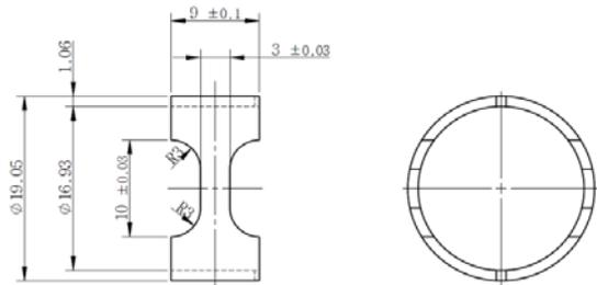
Fig. 1. Geometry of Ring-type circumferential specimen
