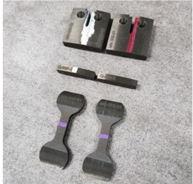
Fig. 5. Various types of specimens with identification numbers after laser marking.
