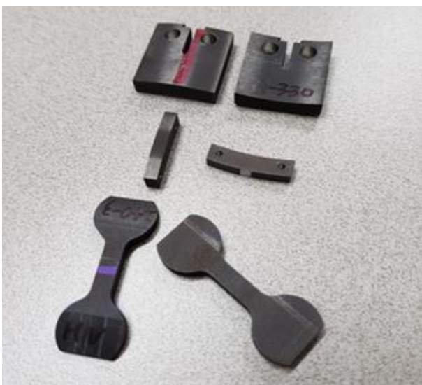
Fig. 2. Unirradiated tube specimens for the laser marking tests
