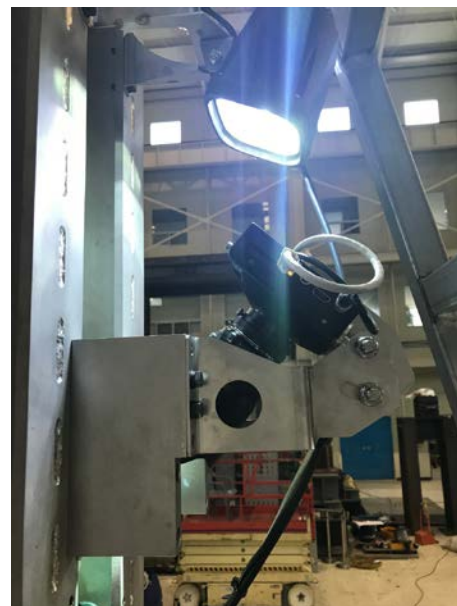
Fig. 5. Photograph of high speed camera installed on test rig #2.
