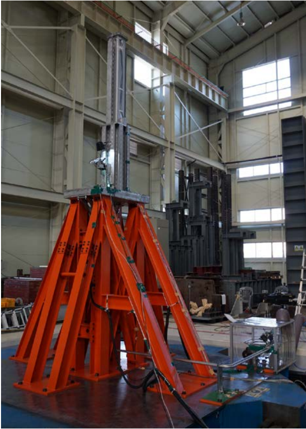
Fig. 6. The photograph of the seismic test rig equipped with SSDM on a tri-axial shaker table.
