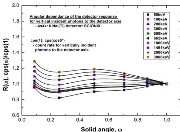
Fig. 4. The angular dependence for the detector response
