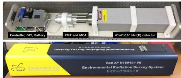
Fig. 1. Environmental radiation survey system
