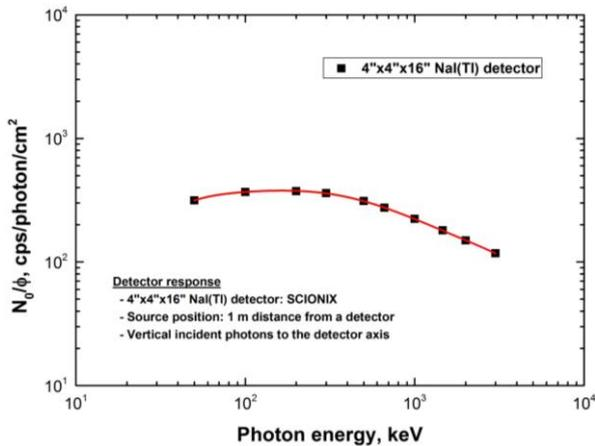
Fig. 3. The detector response of a 4"x4"x16" NaI(Tl) detector for vertically incident photons to the detector axis
