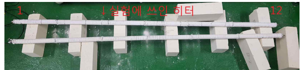
Fig. 6. The electric heater used to measure the segment-wise electric resistance
