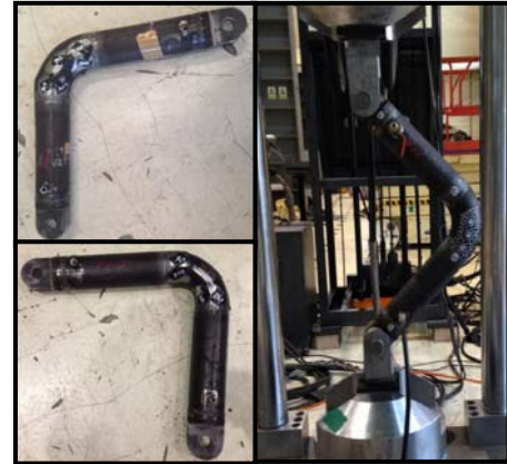
Fig. 2. Cyclic loading test photo
