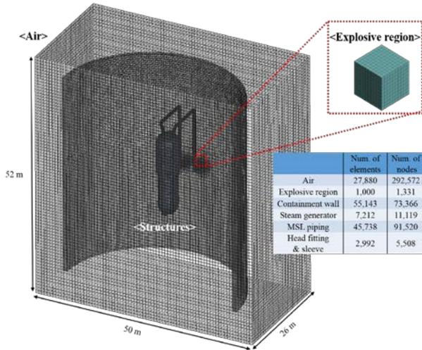
Fig. 1. 3-dimensional FE model for blast wave analysis [4]
