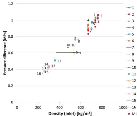
Fig.4. S-CO<sub>2</sub>PE compressor performance test result (pressure difference = P<sub>out</sub>-P<sub>in</sub>) in various inlet density condition
