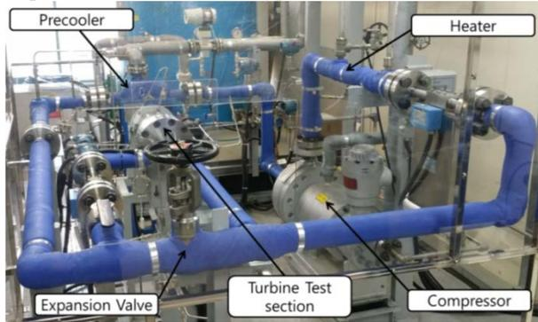
Fig.2. S-CO<sub>2</sub> power cycle demonstration facility (S-CO<sub>2</sub>PE facility)
