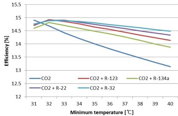
Fig.1. Efficiency comparison of CO<sub>2</sub>+refrigerant cases (R-123 / R-134a / R-22 / R-32) with CO<sub>2</sub> reference case [5]
