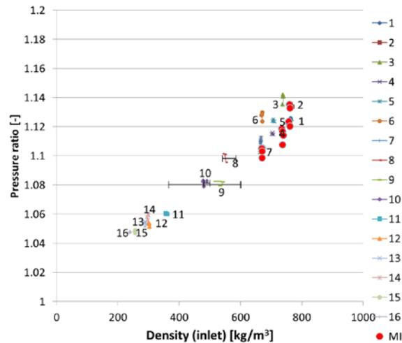
Fig.3. S-CO<sub>2</sub>PE compressor performance test result (pressure ratio = P<sub>out</sub>/P<sub>in</sub>) in various inlet density condition
