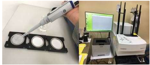
Fig. 1. Preparation of standard samples and measurement equipment (Low background \alpha/\beta counter, 5 XLB)
