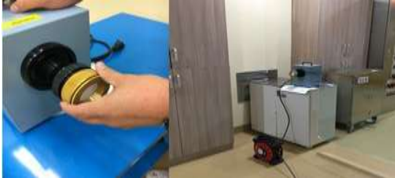
Figure. 2. Replacement of air sampler
