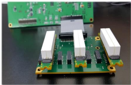
Fig. 5. Sensor module with three sensors (left) and the acquired images (right).
