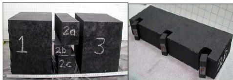
Fig. 7. NBG-10 Block with parts of extracted samples (R, M, F) [6].
