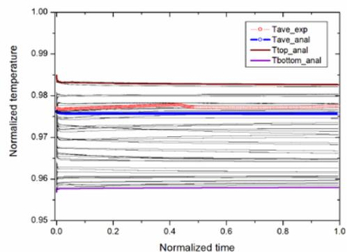
Fig. 6. Estimated temperature distribution in the containment during the test.
