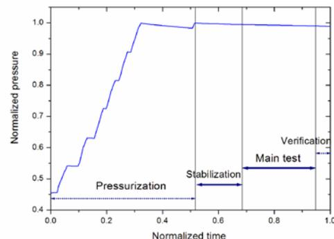
Fig. 1. Containment pressure history during the entire test period in normalized form.
