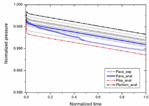
Fig. 5. Calculated containment pressure: comparison with the test data.
