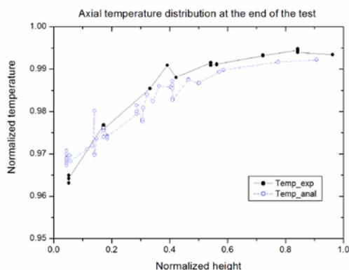
Fig. 8. Calculated axial containment temperature at the end of the test: comparison with the test data
