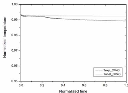
Fig. 9. Calculated local temperature in the top region (CV43: steam generator room): comparison with the test data.
