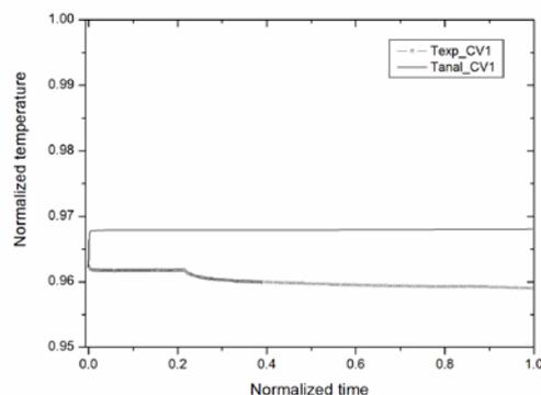
Fig. 10. Calculated local temperature in the bottom region (CV1: access area): comparison with the test data.
