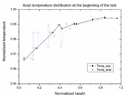
Fig. 7. Calculated axial containment temperature at the beginning of the test: comparison with the test data
