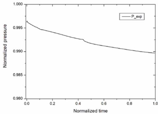
Fig. 2. Measured containment pressure during the test.
