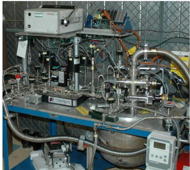
Fig. 1. Self-assaying tritium accountability and containment unit for ITER (STACI) [6].
