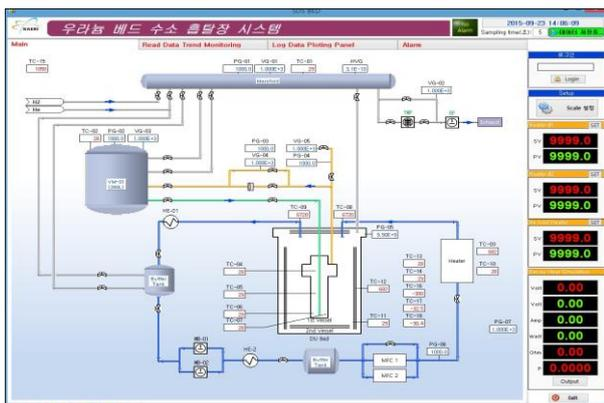
Fig. 7. HMI system for a SDS bed with flowing gas calorimetry [5].
