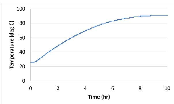
Fig. 4. Temperature change of the SDS bed by heat producing source (approximately 22.5 W).
