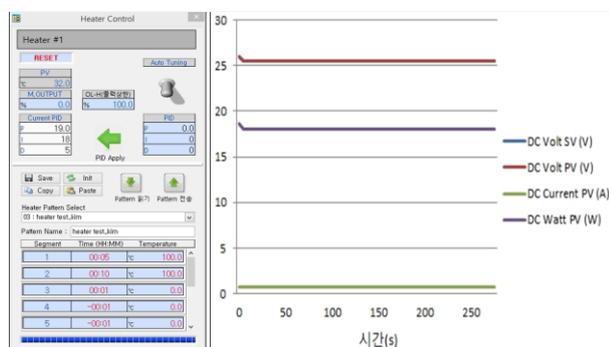
Fig. 8. Heater control system in HMI and simulation results of heater test run [10].
