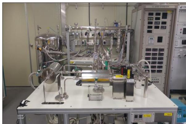
Fig. 6. SDS bed performance test rig with flowing gas calorimetry [5].
