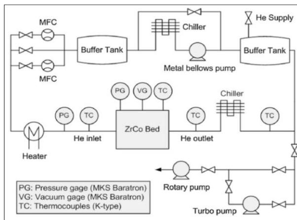
Fig. 5. Schematic diagram of flowing gas calorimetry [9].
