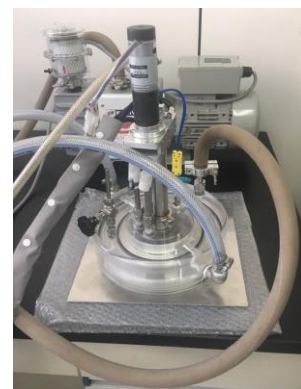
Fig. 2 Photograph of the plating chamber on the Type 304 stainless steel specimen developed by KAERI.
