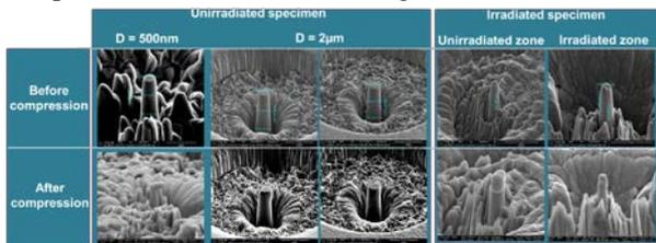
Fig. 4. SEM images of Pillars before and after micro-compression tests
