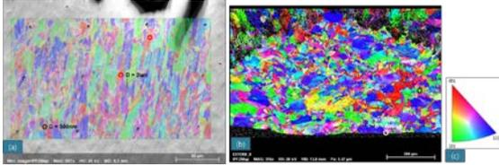
Fig. 3. EBSD maps of (a) unirradiated specimen (vibratory polished), and (b) irradiated specimen (cross-section polished)
