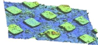
Fig. 6. Measurement the swelling effect by optical coherence tomography
