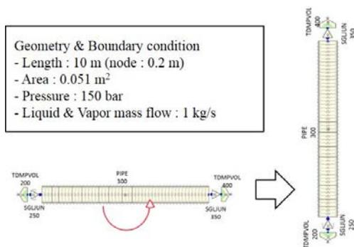
Fig. 2. Concept of horizontal pipe to vertical pipe
