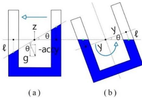
Fig. 6. Concept to calculate water level under (a) translational motion and (b) rolling motion
