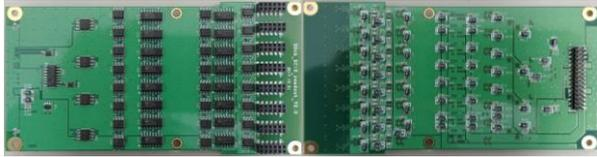
Fig. 4. The fabricated 32-channel charge sensitive readout circuit having eight female headers for mounting photodiode arrays and one male header for communicating to DAQ system. The board size is 135 mm × 71.5 mm.
