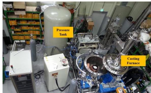
Fig. 1. Engineering-scale injection casting equipment (Max. U-Zr charge: 20kg, installed at KAERI)
