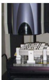
Fig. 3. A Setup for Non-Contacting Cell Size Measurement Device
